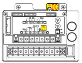
DC model power source terminal plate unit
