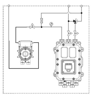
Atmospheric pressure line suction arrangement
