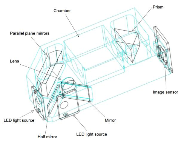
Schematic diagram of an optical interferometric sensor
