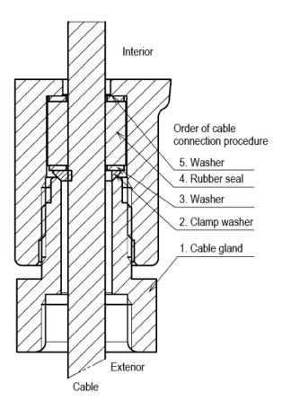
Tighten cable glands to a torque of at least 40 N□m.
