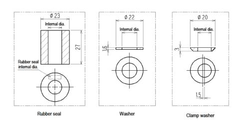
Table 1. External cable inlet parts diameters
