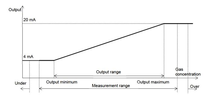
A preset special output value is output if an abnormality (FAILURE) is detected by self-diagnosis or during function checking (FUNCTION CHECK) (mainly in setup mode).
