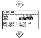
Use the ▲ and ▼ keys and SET key to enter and confirm the gas concentration for outputting 20 mA.
